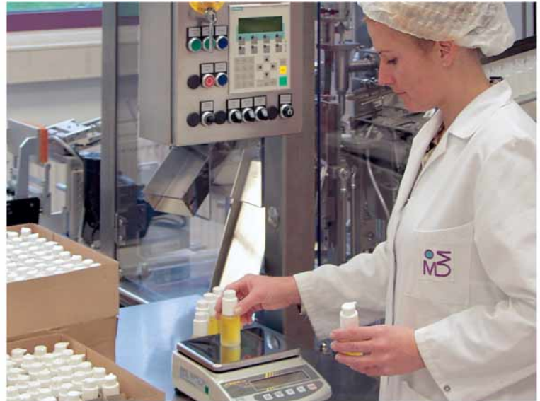
Checkweighing application in the cosmetics industry.
