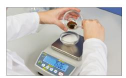
With the **recipe function** you can weigh the different ingredients of a mixture. As a check, you can also call up the total weight of all the ingredients
