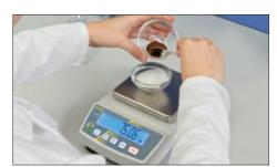
With the **recipe function** you can weigh the different ingredients of a mixture. As a check, you can also recall the total weight of all the ingredients
