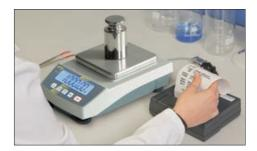
GLP/ISO record keeping of weighing data, balance adjustment, etc. with date, time and identification no... Ideal for monitoring and documenting your processes in accordance with your quality management system
