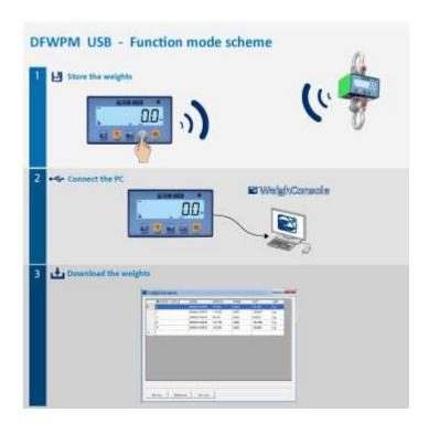
DFWPM has to be coupled with scales or crane scales fitted with optional radio module.
